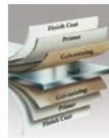
Panels are preprimed inside and out to inhibit rust. Hot-dipped, galvanized steel is painted with primer and given a tough oven-baked polyester top coat to provide the most rust-resistant steel door available. Ten-year warranty against rust-through.
